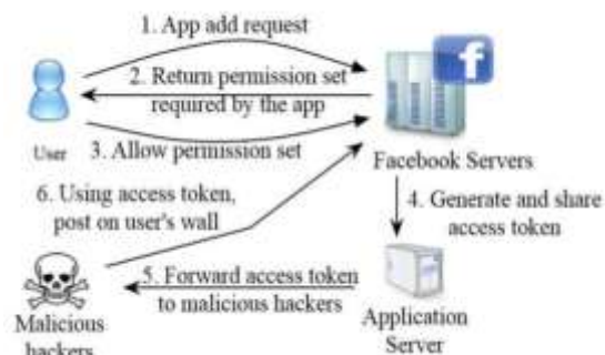
Fig 1: Steps involved in hackers using malicious applications to get access tokens to post malicious content on victims' walls.
