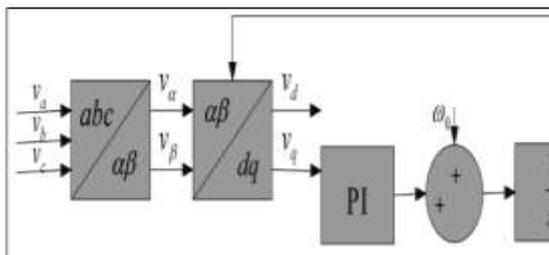
Figure.1.3. Block diagram of synchronous reference frame PLL
