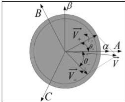
Figure.1.5. Voltage vector decomposition (unbalanced voltage)
