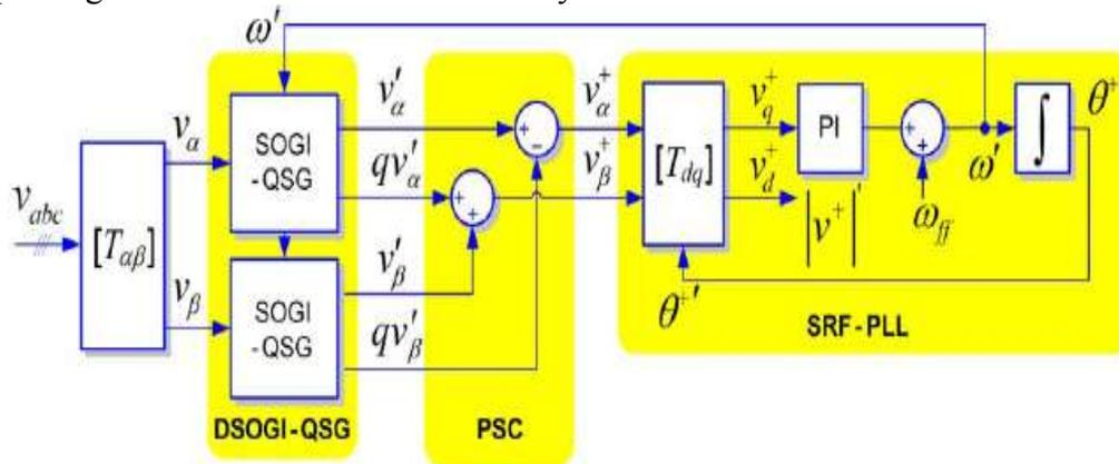
Figure.2.4. DSOGI-PLL block diagram.
