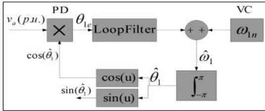
Fig.1.2. Block diagram of linear PLL
