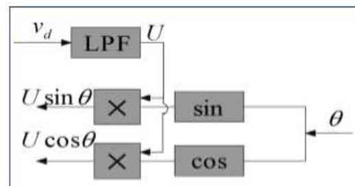
Figure.1.4. Synthesis circuit used in DSRFPLL
