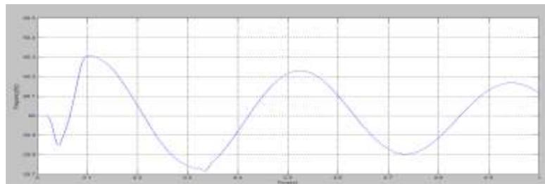
Figure.5.15. Frequency value of DDSRF PLL under 1-ph sag
