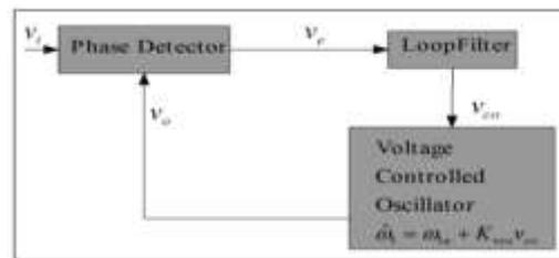
Fig.1.1. Block diagram of PLL
