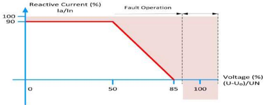
Figure.2.2.REE voltage support requirement in the event of grid fault.
