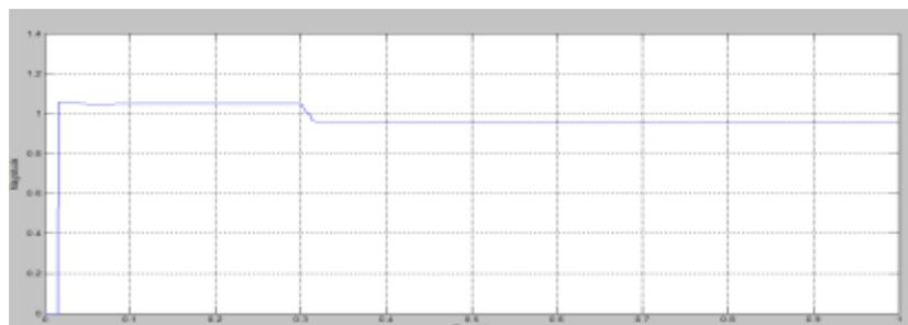
Figure.5.13. Voltage magnitude of DDSRF PLL under 1-ph sag(Type-c)
