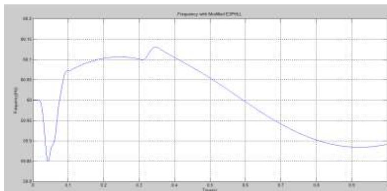
Figure.5.35. Frequency value of 3-ph EPLL under 3-ph sag
