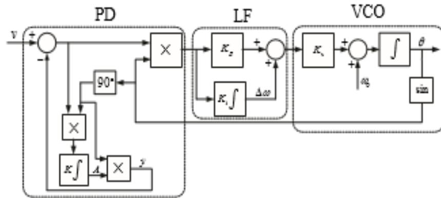
Figure.1.9. Block diagram of single phase EPLL
