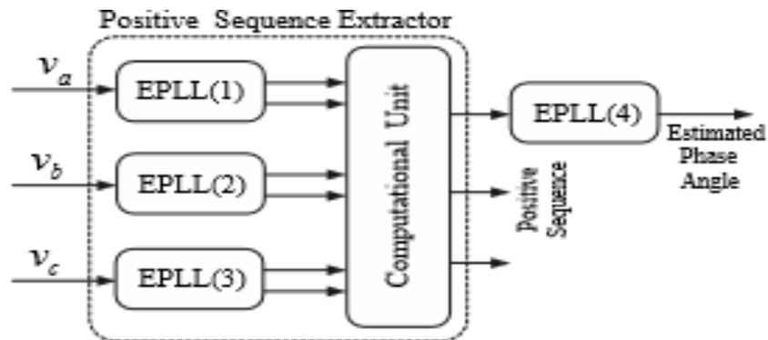
Figure.1.10. Block diagram of 3-PH EPLL
