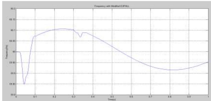
Figure.5.41. Frequency value of 3-ph EPLL under 1-ph sag
