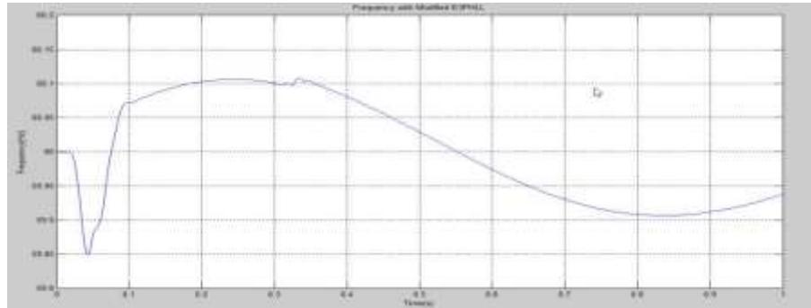
Figure.5.44. Frequency value of 3-ph EPLL under 2-phase sag-2
