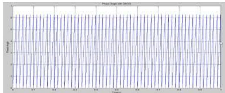
Figure.5.30. Phase value of DSOIG PLL under 2-phase sag-2
