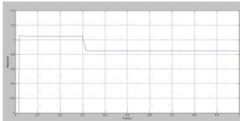
**Figure.5.10. Voltage magnitude of DDSRF PLL under 2-phase sag-1(Type-B)**
