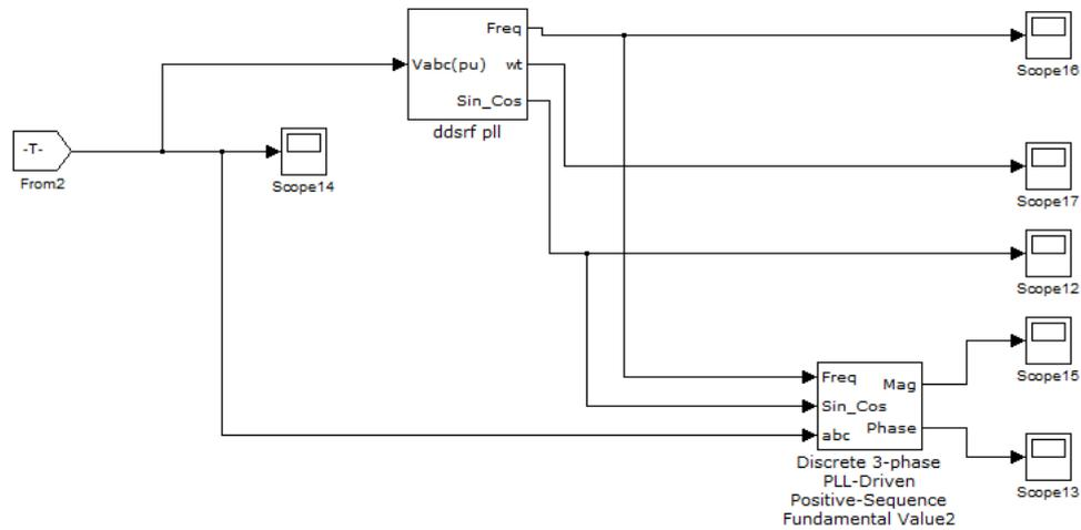
5.6. Block diagram for DDSRF-PLL
