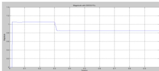
Figure.5.23. Voltage magnitude of DSOIG PLL under 2-phase sag-1
