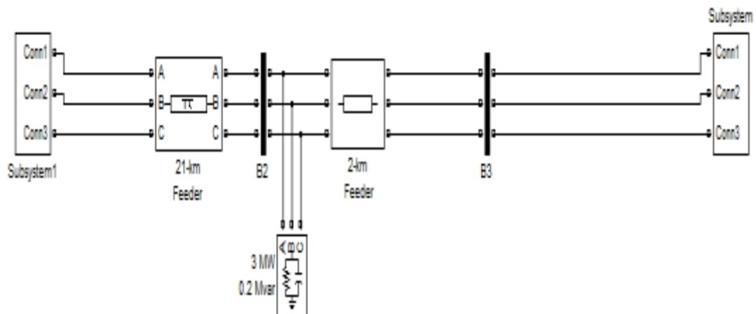
Figure: 5.1.BLOCK DIAGRAM OF VOLTAGE SAGS
