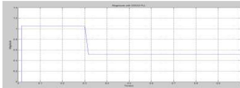
Figure.5.20. voltage magnitude of DSOIG PLL under 3-ph sag
