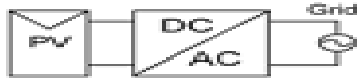
Fig 5. A single power processing stage that handles the MPPT, voltage amplification, and grid current control
