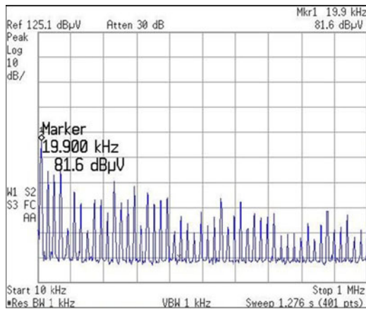
Fig. 15. Spectrum of the CM voltage with the active filter without feed-forward signal by CM current estimation.
