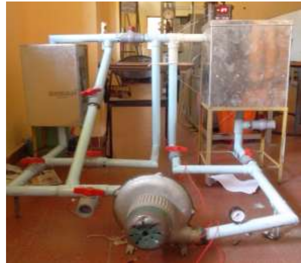
Figure 5. Air flow path of seed drying
