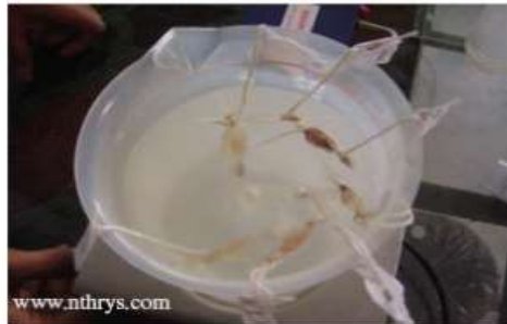
The process of Dialysis Precipitated plasma samples in Dialysis bag dialyzing against Phosphate buffer
