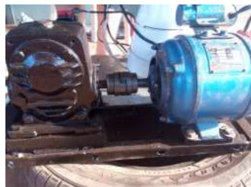
Figure2. Arrangement of Gear Box and Motor
