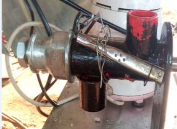
Figure7. Pressing Barrel with Heating Unit
