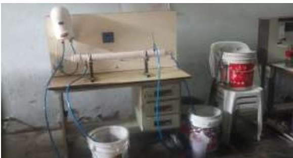
Fig 3: Experimental set up of Heat exchanger
