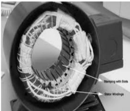
. BLDC motor stator construction
