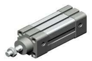
In pneumatic system, the piston rod in cylinder is moved by the supply of compressed air which is supplied through the solenoid operated 5/2 way directional control valve. The cylinder A and B ports are connected to the 5/2 way solenoid D.C. Valve with 6/8mm PVC tube. The 6mm connector is used to connect this cylinder port and D.C valve. The minimum air pressure required is 5 to 6bar. The figure shows the cross section view of double acting cylinder.
