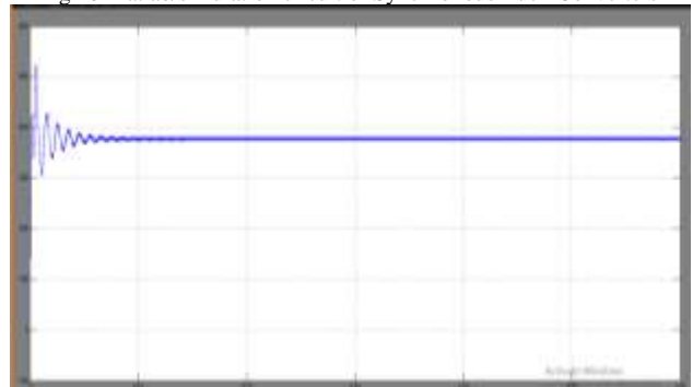
Fig 11 simulation wave form of buck converter output voltage
