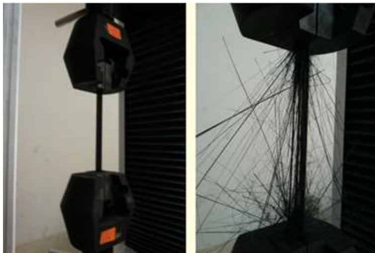
a)The specimen before test b) The specimen after Failure
