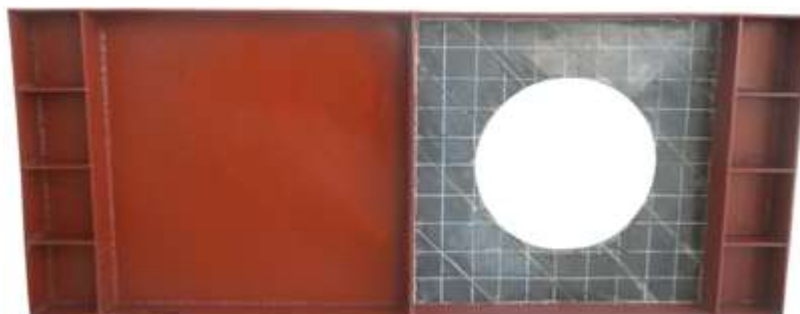
D).Plate girder PGOC2
