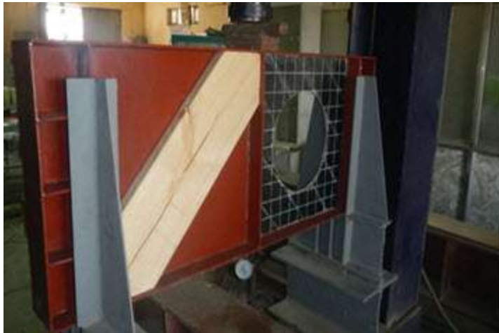
Figure (4): Test setup for plate girder specimen
