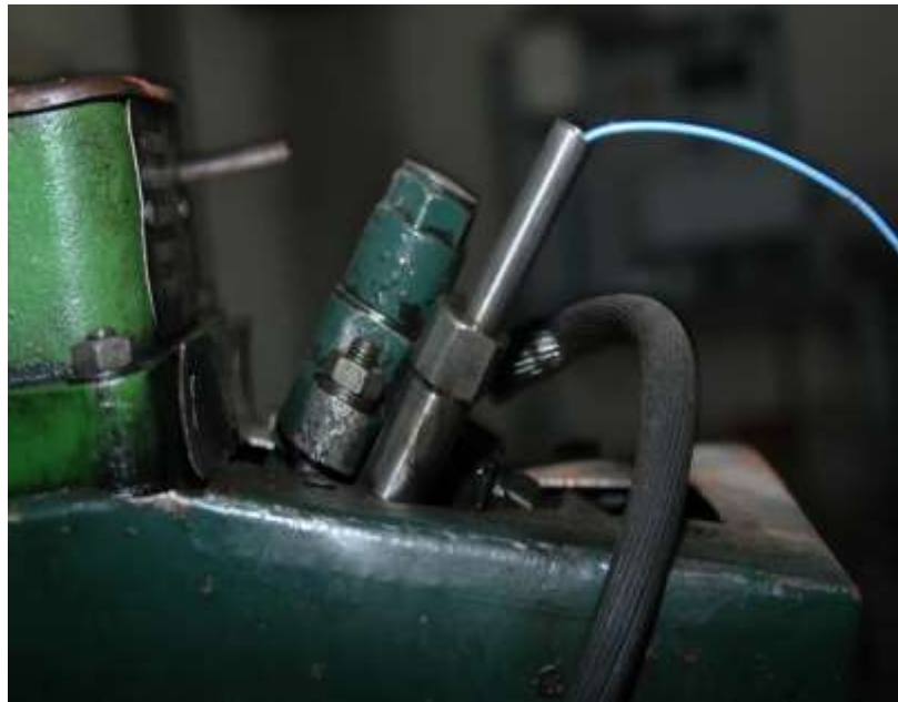
Fig. 3.7: Pressure transducer in mounted position
