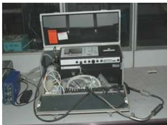
Fig. 3.3: MRU delta 1600 L exhaust gas analyzer
