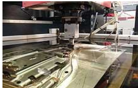
Figure 2: Wire-Cut EDM machine tool
