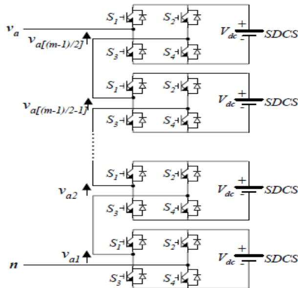
Fig 2. Single-phase structure of a multilevel cascaded H-bridges inverter
