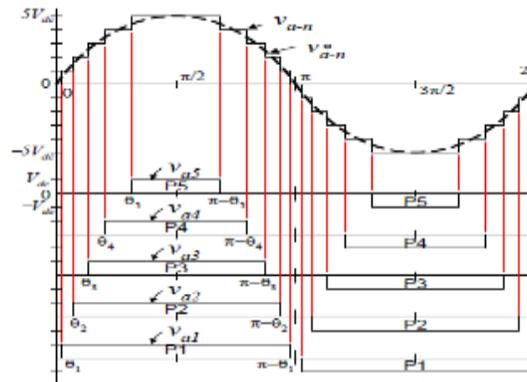
Fig 3. Output phase voltage waveform of an 11-level cascade inverter with 5 separate dc sources.
