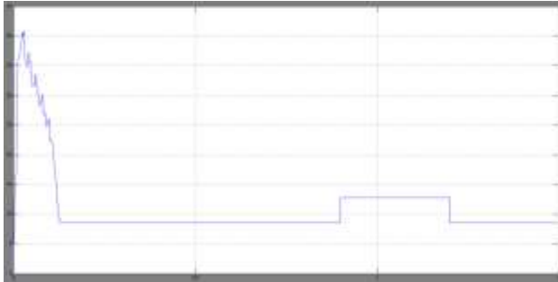
Fig.17. simulation results for compensation current of statcom
