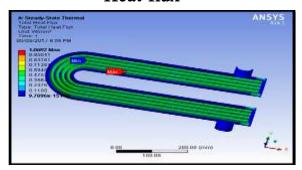
According to the contour plot, the maximum heat flux at inside the tubes because the nano fluid passing inside of the tube. So we are applying the temperature inside of the tube and applying the convection except inside the tubes. Then the maximum heat flux at inside the tubes and minimum heat flux at heat exchanger casing and outside of the tubes.
