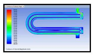
According to the above contour plot, the maximum velocity magnitude of the heat exchanger at hot fluid inlet and minimum velocity magnitude at cold fluid outlet.
