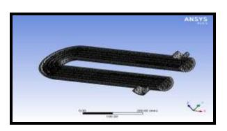
Finite element analysis or FEA representing a real project as a "mesh" a series of small, regularly shaped tetrahedron connected elements, as shown in the above fig. And then setting up and solving huge arrays of simultaneous equations. The finer the mesh, the more accurate the results but more computing power is required.
