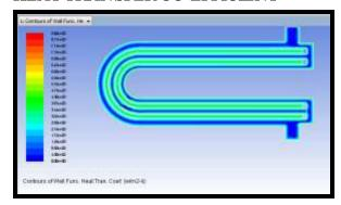
According to the above contour plot, the maximum heat transfer coefficient of the heat exchanger at inside the tubes and minimum heat transfer coefficient inside the heat exchanger casing. According to the above contour plot, the maximum heat is  $8.60 \text{w/m}^2 - \text{k}$ transfer coefficient and minimum heat transfer coefficient is  $4.30e+02w/m^2-k$ .
