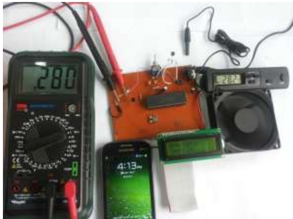
Fig. 10 Calibration process using the voltmeter and the thermometer
