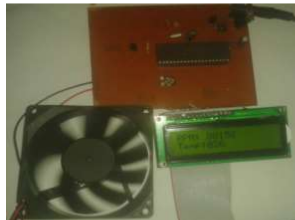
Fig. 9 Hardware circuit of fan speed control system
