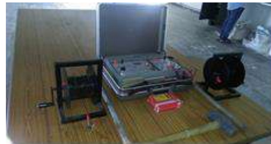
Fig 1. Electrical Resistivity Meter along with Winches and Probes.
