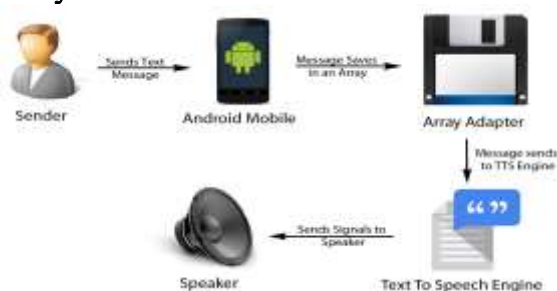
Fig. System Architecture
