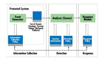
Logs are used to collect information about network activities, which are analyzed. Attacks are detected based on the rule set. Then, appropriate response is taken to prevent or mitigate attacks.
