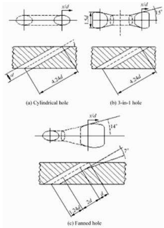
Fig.4.1. Geometrics of three film cooling holes.
