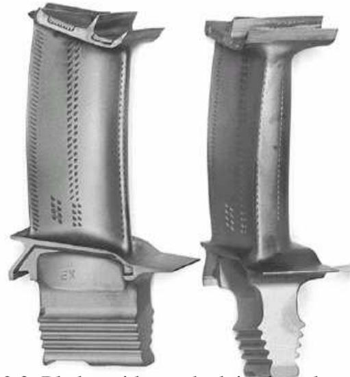
Figure 2.3: Blades with attached tip shrouds.
