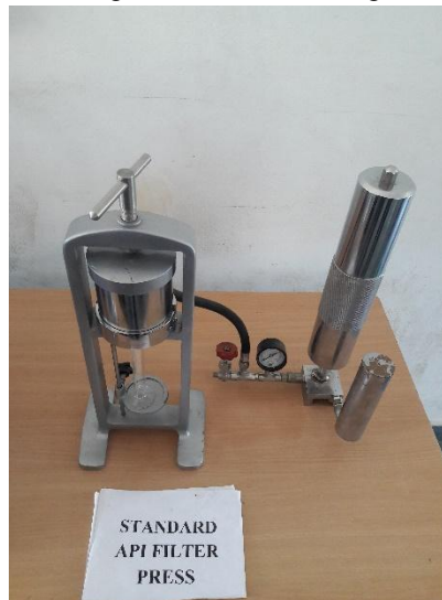
Fig.15: Filter cake thickness is also measured and must never exceed 2 mm.
