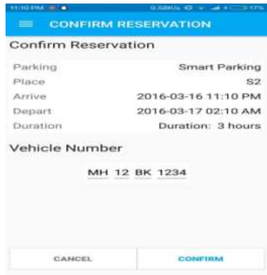
Figure 5. Android app prototype shows the details of reservation before confirming the slot
