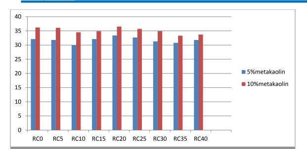
Result analysis- According to results there is a 13% increase in strength for RC20 cube when we are adding metakaolin by weight of 10% of cement as a admixture and in RC20 20% natural aggregates are replaced by recycle coarse aggregates.
