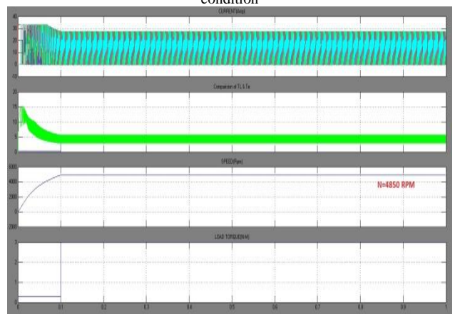
Fig.16. shows the simulated waveforms of current, load torque, speed and Te under 5000 rpm speed using fuzzy controller at 3/4 th load condition
