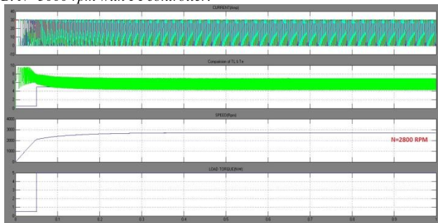
Fig.11. shows the simulated waveforms of current, load torque, speed and Te under 3000 rpm speed using PI controller at full load condition
