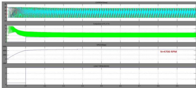
Fig.9. shows the simulated waveforms of current, load torque, speed and Te under 5000 rpm speed using PI controller at 3/4 th load condition
