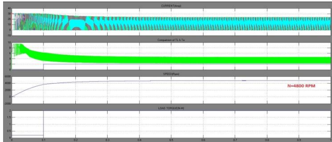
Fig.10. shows the simulated waveforms of current, load torque, speed and Te under 5000 rpm speed using PI controller at half load condition
