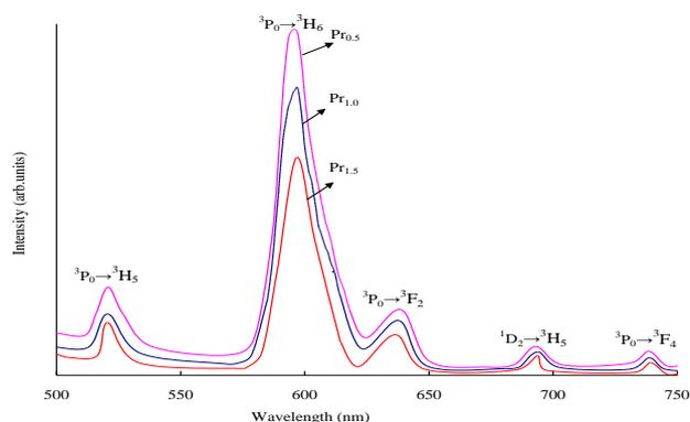
Fig.8 Photoluminescence spectra for ZnF<sub>2</sub>-PbO-P<sub>2</sub>O<sub>5</sub>: Pr<sup>3+</sup> glasses recorded at room temperature ( $\lambda_{exc}$ =440 nm)
