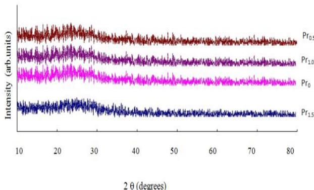
Fig. 5 X-Ray diffraction pattern of ZnF<sub>2</sub>-PbO-P<sub>2</sub>O<sub>5</sub> glasses doped with different conc. of Pr<sub>2</sub>O<sub>3</sub>.
