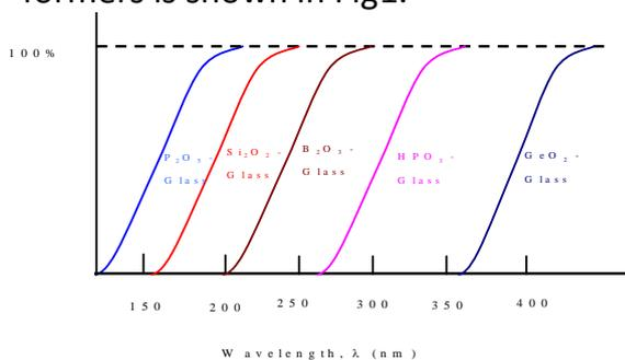
Fig.1 Comparative diagram of the UV edges of various glass formers.
