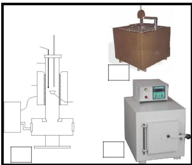
**Fig.2(a)** Schematic sketch high temperature furnace and the photographs of ( b) Melting furnace (c) Annealing furnace
