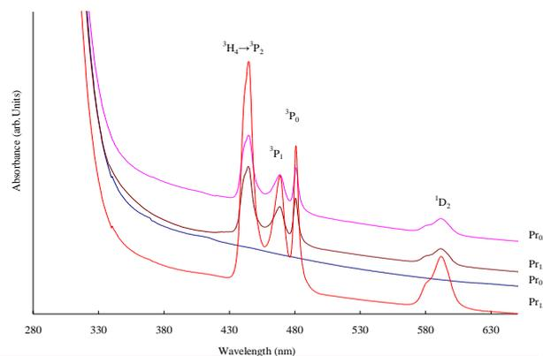
Fig.7 Optical absorption spectra for ZnF<sub>2</sub>-PbO-P<sub>2</sub>O<sub>5</sub> glasses doped with different conc. of Pr<sup>3+</sup> ions.
