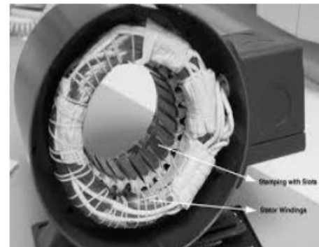
Fig.4. BLDC motor stator construction
