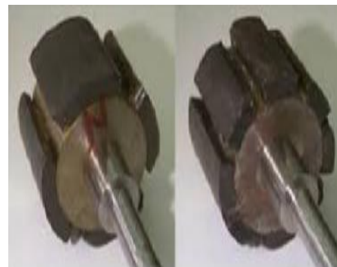
Fig.5. BLDC motor Rotor construction.
