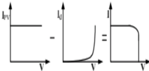
Fig.6.Characteristics I-V curve of the PV cell.
