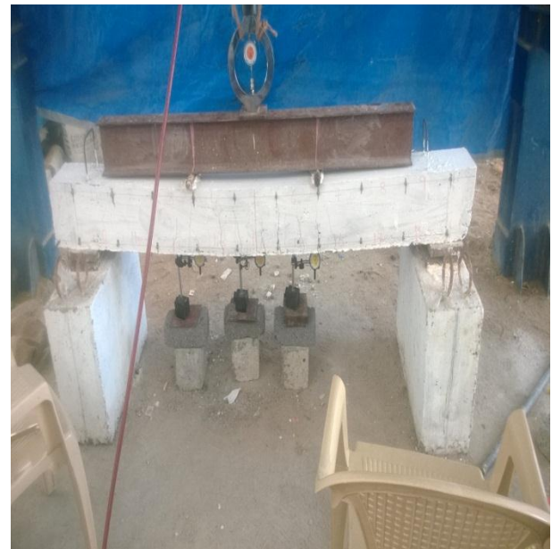
Fig 4 CNBM beam crackings.
