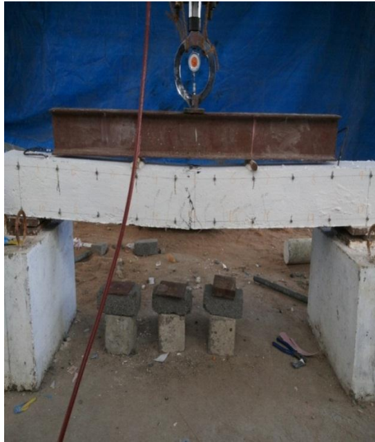
Fig 5 HYBM-1 cracking pattern
