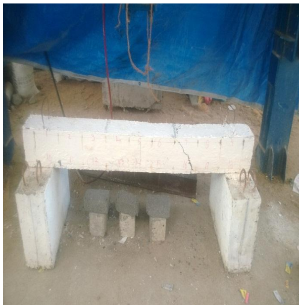
Fig 6 HYBM-2 Cracking pattern
