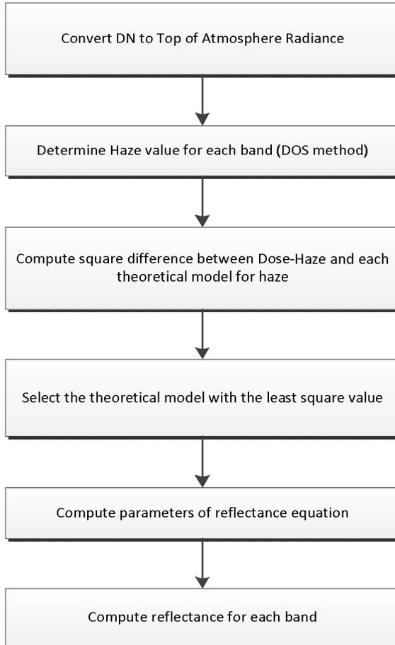
Figure 2 Flow chart for computing reflectance of 8-band images
