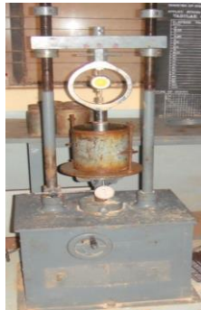
Fig 4. California bearing ratio testing machine and the specimen undergoing testing.
