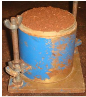
Fig 1. Preparation of sample by IS Heavy Compaction to determine Maximum dry density and Optimum moisture content
