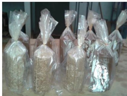
Fig 3. Curing of samples prepared for Unconfined Compression Test
