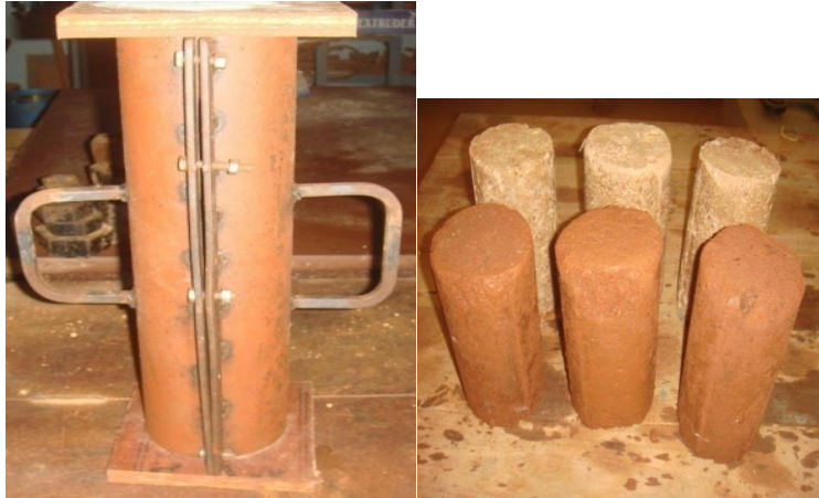
Fig 2. Mould assembly compressed under UTM and samples obtained for UCS Testing
