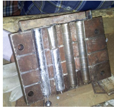
Figure 2. Inside Die when casted
