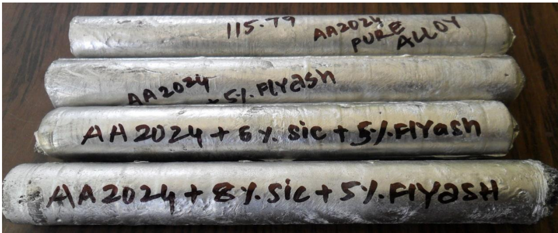
Figure 3. Specimens after casting Specimen Compositions:
