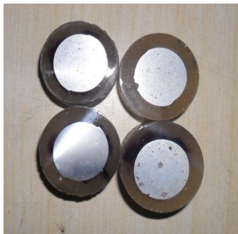
Figure 4. Mounted Specimens for Microstructures
