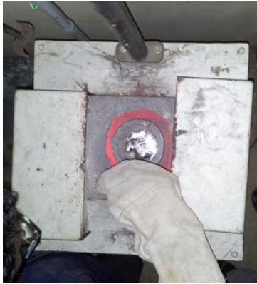
Figure 1. Crucible in Stir casting machine
