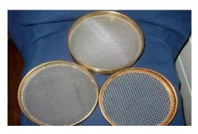
Weigh roughly 10g of concrete to the closest 0.01g and place it on the strainer.
