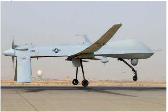
At present the most commonly used military robot is the unmanned aerial vehicle IAI Pioneer and RQ-1 Predator. These robots can be armed with Air-to-ground missiles.
