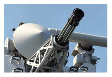
Goalkeeper – As far as the current use of robots in military is concerned, we cannot leave behind Goalkeeper. This military robot is a Dutch close-in weapon system that helps to defends ships from incoming missiles as well as ballistic shells. This system generally comprises of auto cannon and advanced radar that tracks incoming fires. It is an automatic system that can be also be deployed to protect
