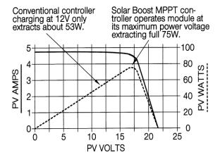
Rather than simply connecting the module to the battery, the patented MPPT system in a
