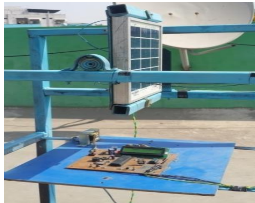
Figure 6: single axis tracking solar panel at ( -86.85 tracking angle with respect to the ground
