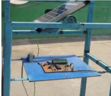
Figure 9: single axis tracking solar panel at (45° tracking angle with respect to the ground
