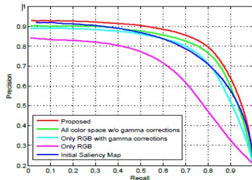
Fig.4. Comparison of precision-recall curves of proposed initial map And results based on different color transforms on the MSRB Dataset
