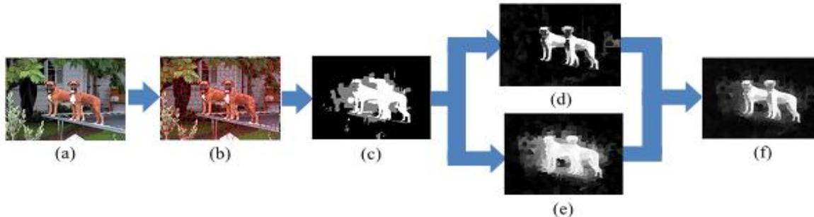
Fig.1. Overview of our algorithm: (a) Input image. (b) Over-segmentation to super pixels. (c) Initial saliency trimap. (d) Global salient region detection via HDCT. (e) Local salient region detection via random forest. (f) Final saliency map
