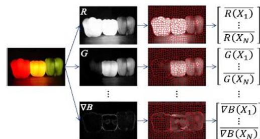
Fig.2.HDCT concatenate different nonlinear RGB transformed color space representations to form a high-dimensional feature vector to represent the color of a pixel.
