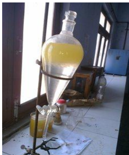
Fig. Separation of water and biodiesel in Separating funnel after Water Washing
