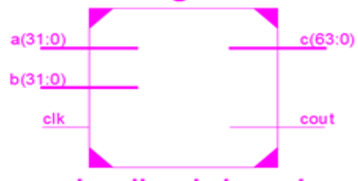
FIG 5. RTL SCHEMATIC OF DUAL MODIFIED ADAPTIVE MULTIPLIER.
