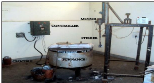
Fig 1: Aluminium Stir Casting Furnace
