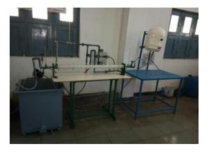
The experimental setup consists of two concentric tubes in which fluids pass. The hot fluid is hot water, which is obtained
