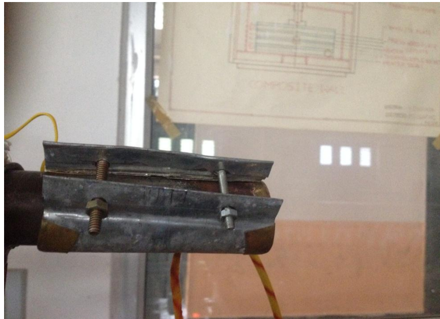
Figure 4 Heater is fitted to the heat pipe in the evaporator section
