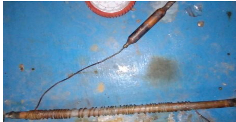
Figure 3 Heat Exchanger like set up
