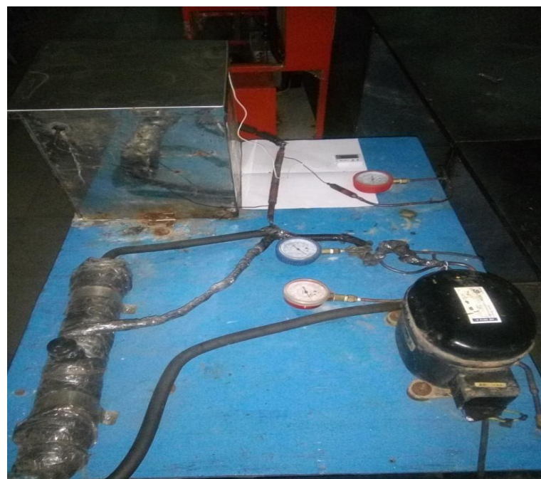
Figure 4 Complete set up with Heat Exchanger
