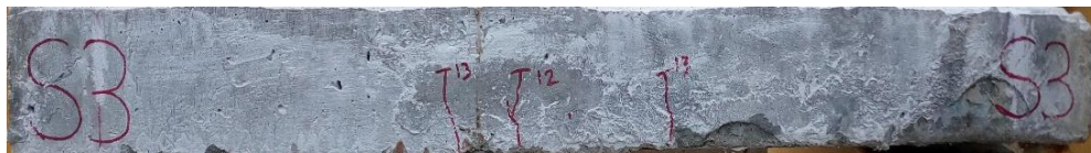
Fig. 5.10 Modes of cracks for S3 at failure
