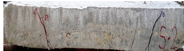
Fig. 5.9 Modes of cracks for S2 at failure
