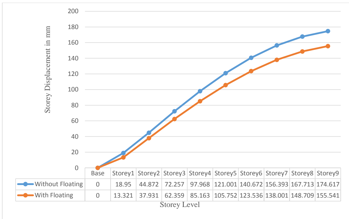
Fig.5.3 Storey displacement in Zone III Soil II Graph for with and without Floating Columns
