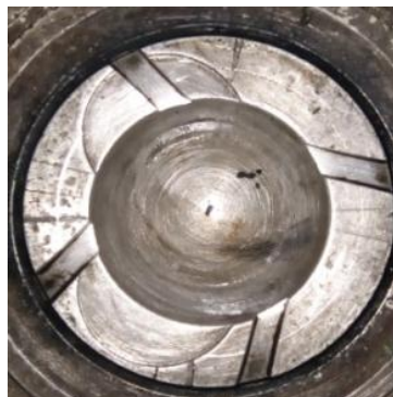
Figure 3 Tangential grooves on piston
