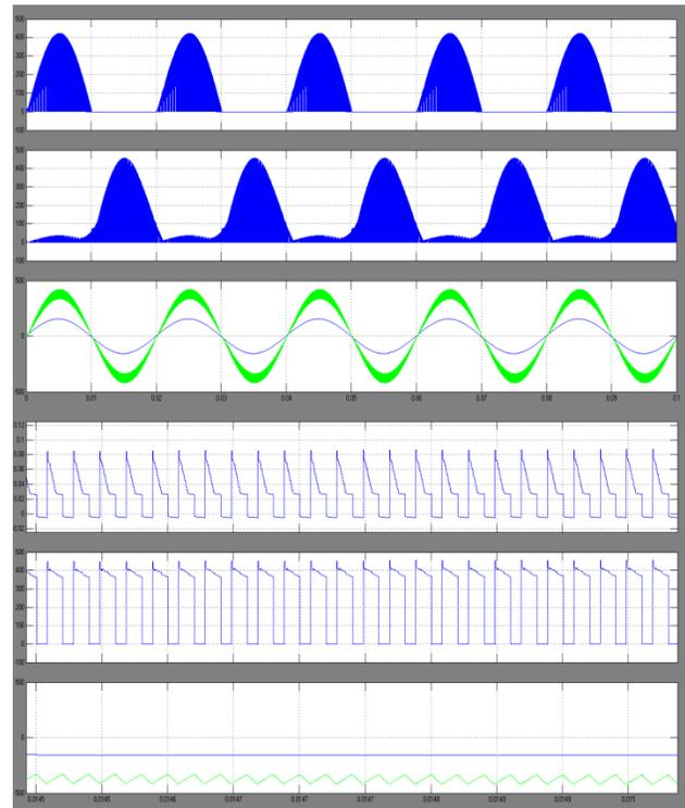
Fig.10 Experimental results with resistive load when  $D=0.4$ .
