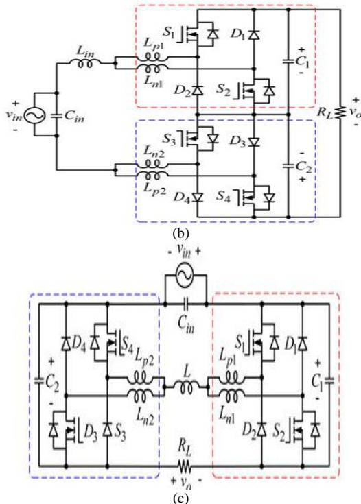
Fig.2. Proposed single-phase ac-ac converters. (a) Buck type. (b) Boost type. (c) Buck-boost type.
