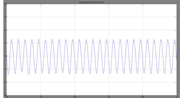
Fig.17 Torque characteristics of the induction motor
