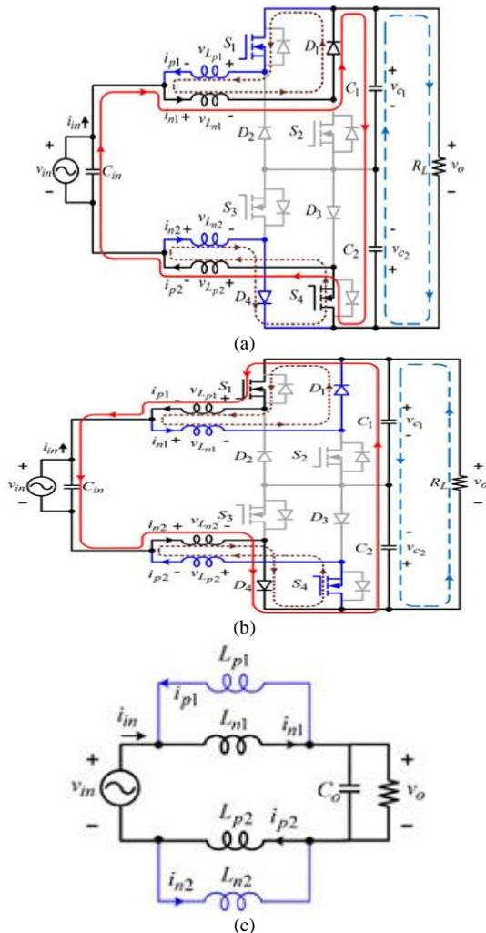
Fig.5. Mode 2 of the proposed boost type ac-ac converter.
