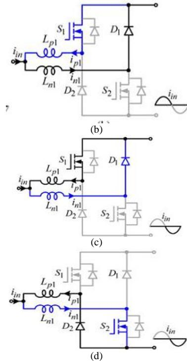
Fig.3. Conduction states of the proposed boost-type ac-ac converter. (a)  $i_{in} > 0$  and  $S_2$  on. (b)  $i_{in} > 0$  and  $S_2$  off. (c)  $i_{in} < 0$  and  $S_1$  on. (d)  $i_{in} < 0$  and  $S_1$  off.
