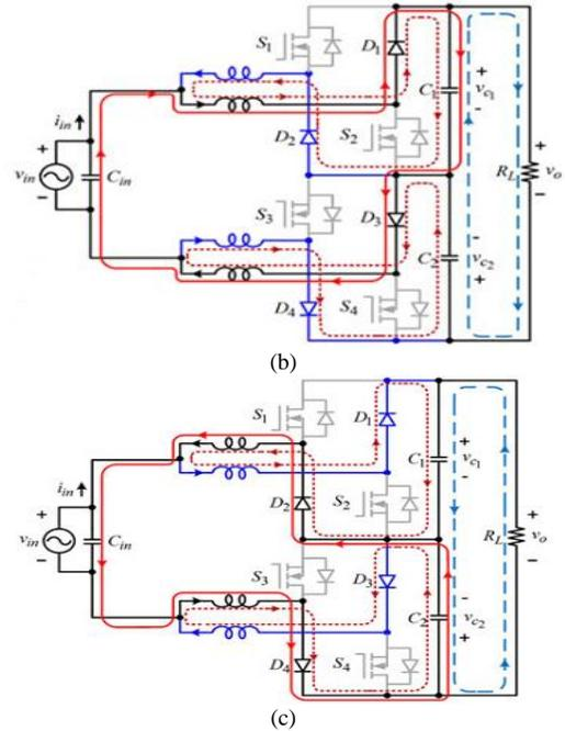
Fig.6. Operation of the proposed boost type ac-ac converter during dead time. (a) Dead time. (b)  $v_{in} > 0$ . (c)  $v_{in} < 0$ .
