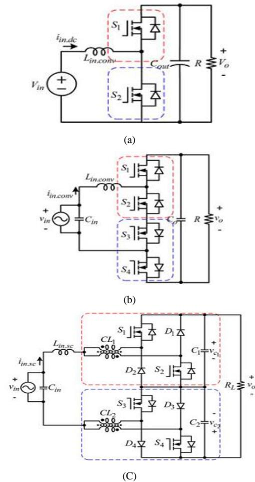
Fig.1. Boost-type dc–dc and ac–ac direct PWM converters. (a) Traditional dc–dc converter. (b) Traditional ac–ac converter. (c) SC ac–ac converter [13]
