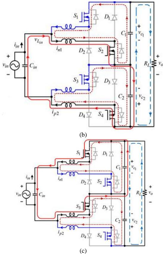
Fig.7. Operation of the proposed boost type ac-ac converter during overlap time. (a) Overlap time. (b)  $v_{in} > 0$ . (c)  $v_{in} < 0$ .
