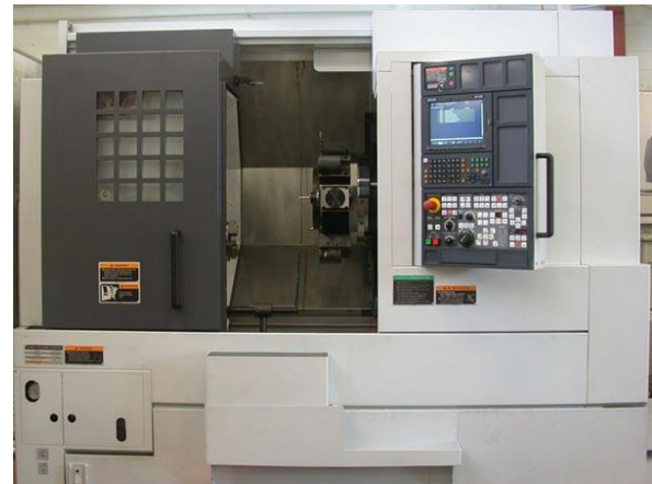
Fig shows 4-axis CNC MORI SIEKI turning machine
