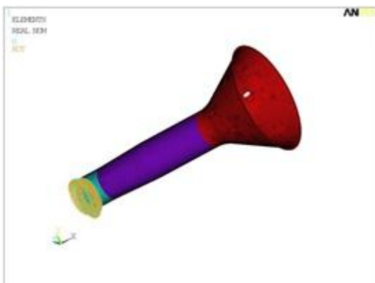
Fig Boundary conditions for Modal analysis
